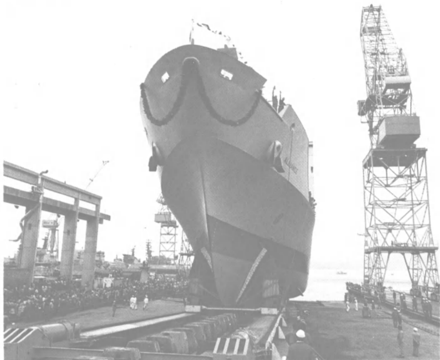
Research ship Alliance is under construction at Muggiano yard of Fincantieri in La Spezia. Sophisticated vessel will be powered by GMT/AEG diesel-electric plant.
