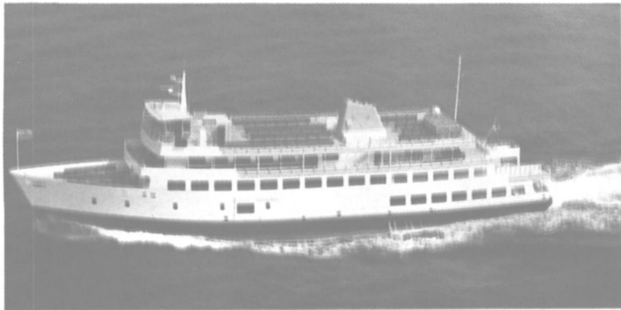
The Anna C. features a triple-screw propulsion plant with three Cummins diesel engines coupled to Twin Disc gears. The vessel's primary function is to provide ferry service from New London, Conn., to Block Island, R.I.
