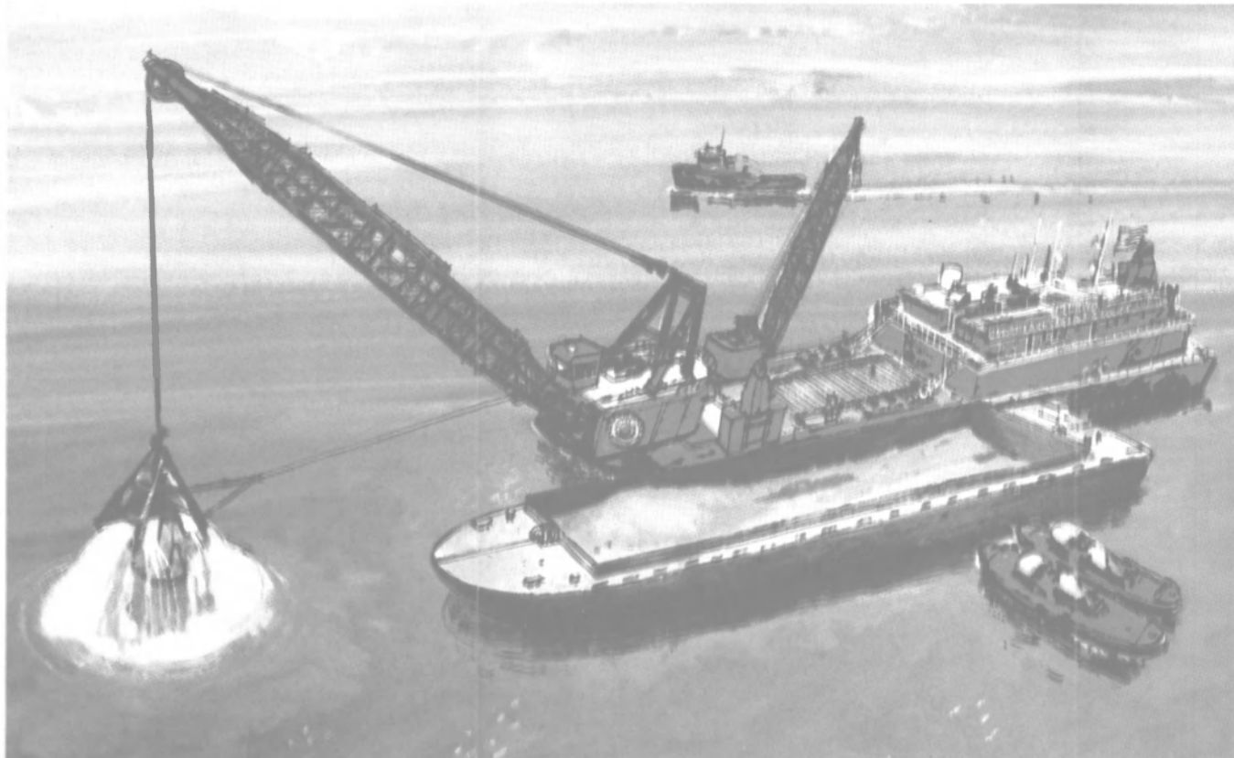
Artist's rendering shows dredge Chicago in clamshell mode with barge alongside.
