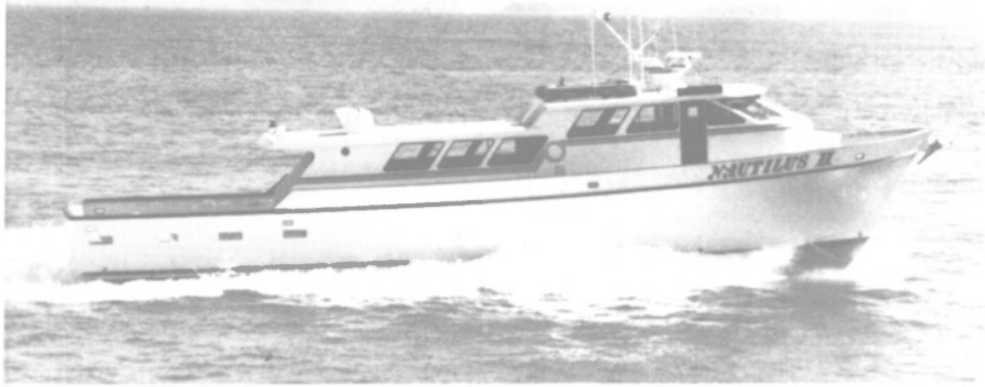
Excursion/fishing vessel Nautilus II built by Westport Shipyard is powered by twin Detroit Diesel 12V92N engines with total output of 1,020 bhp for top speed of 21 knots.
