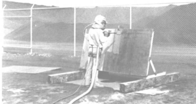
COPPER BLAST (in use here) has very little dust, is low in free silica, cuts 30-50% better than lower-quality slag abrasives and up to four times better than many silica sands.
