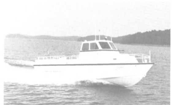
Fast Parasail Training Craft built for Air Force by MonArk Boat is powered by twin 435-bhp Detroit Diesel engines providing speed of about 30 mph.
