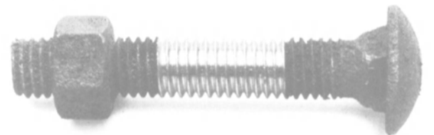
After being submerged in salt water for 12 months, portions of bolts covered with Never-Seez remained free of corrosion.
