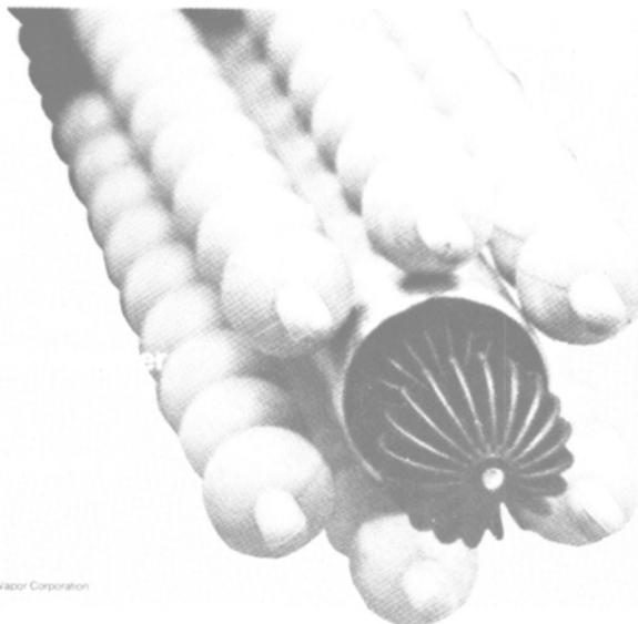
The heart of the SPHERE MATRIX Technology consists of nesting the tubes in a regular matrix of solid spheres around the outside and utilizes fluted spheres, properly spaced, on the inside. The spheres interrupt the boundary layer growth and thereby enhance the heat transfer performance.
