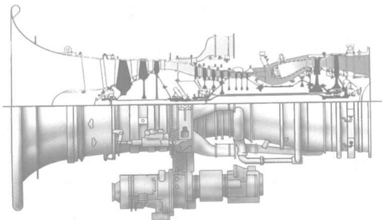
General Electric's LM1600 Simple Cycle Gas Generator.
