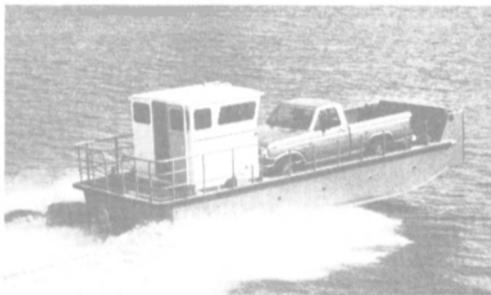
MonArk's 30-foot transportation barge is powered by twin AQAD40/290 Volvo I/O diesels (165 hp each).
