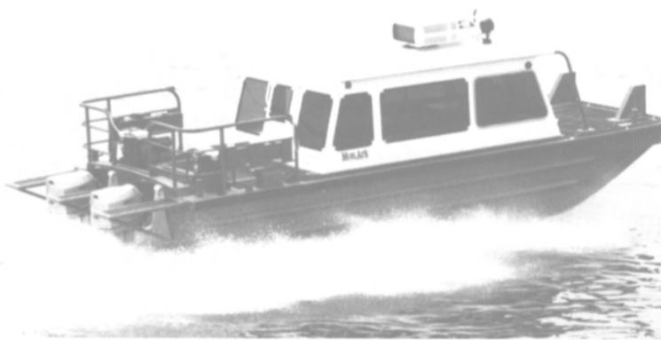
MonArk's new 26-foot survey boat is powered by two Outboard Marine Corp. "sea drives" rated each at 155 hp, yielding a top speed of approximately 32 knots.
