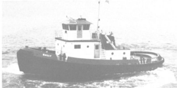
The twin-screw, 360°-rotating-nozzle, ship-docking tug Sally is powered by two G.M. Detroit Diesel Allison engines rated 900 shp at 2,400.
