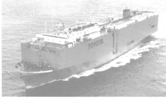
The Overseas Joyce has a total of 13 car decks and can carry a total of 5,300 automobiles.
