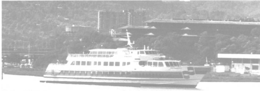
The M/S San Francisco's overall performance improved when it was repowered with two Detroit Diesel 16V-149TIB marine diesels.
