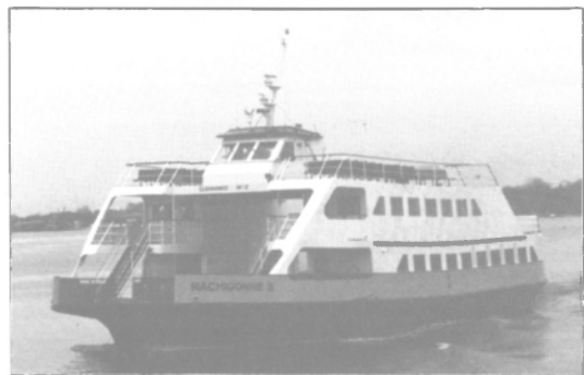
MACHIGONNE II OCTOBER 1987 122'x36'x9' Steel Passenger/Auto Ferry Owner: Casco Bay Island Transit District, Portland, ME
