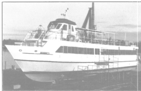
LA NINA DECEMBER 1987 92'x22'x5' Aluminum Passenger Ferry Owner: Puerto Rico Ports Authority
