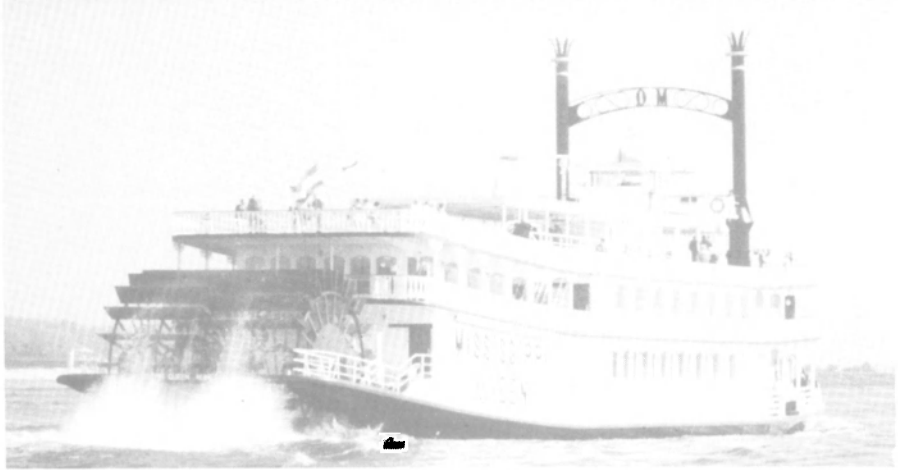
The Mississippi Queen is Europe's first newbuilding based on the famous Mississippi paddle steamers. With a length of 203½ feet and a beam of 37½ feet the vessel can hold up to 1,000 passengers. The paddlewheel, 23 feet in diameter and 26 feet wide, has a hydrostatic drive. Power is delivered by two Deutz MWM 234 series engines arranged in the forebody.
