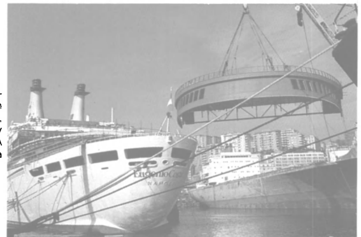
At left: the flagship of Costa Lines, the Eugenio Costa, recently underwent a $20-million conversion at the Mariotti yard in Genoa, Italy. At right: Conversion work underway on the Eugenio Costa at the Mariotti yard. A large section was mounted aft to house a 600-seat theatre.
