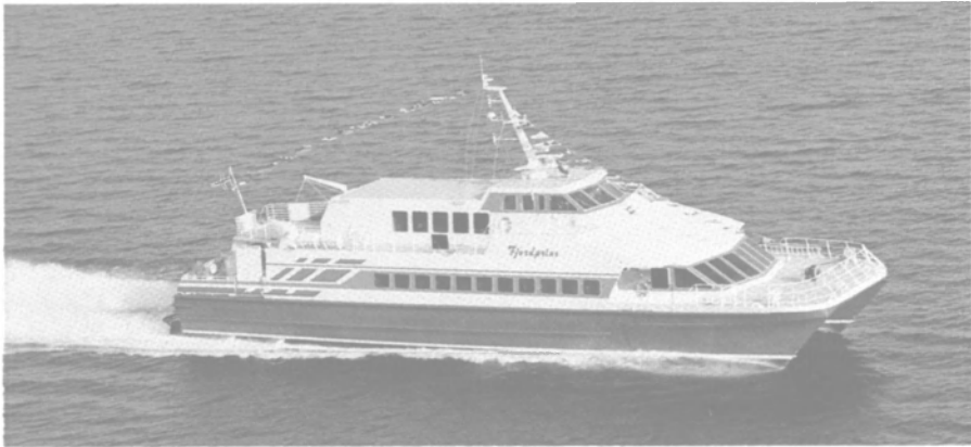
The high-speed catamaran Fjordprins is propelled by two KaMeWa waterjets. Her main engines are MTU and reduction gears, ZF. She can reach 38 knots.
