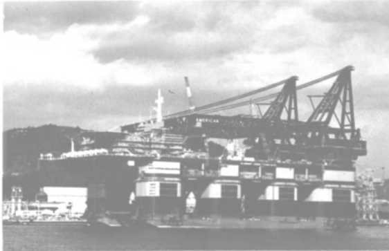
Photos (L to R): The general cargo ship Madang Coast was the first ship built to ABS Class in the People's Republic of China; the world's largest mobile offshore unit, the ABS-classed McDermott Derrick Barge No. 102, is a twin-hull, column stabilized-type with a length of 625 feet; and the 105-foot tugboat Bergantin was built in Venezuela to ABS class.
