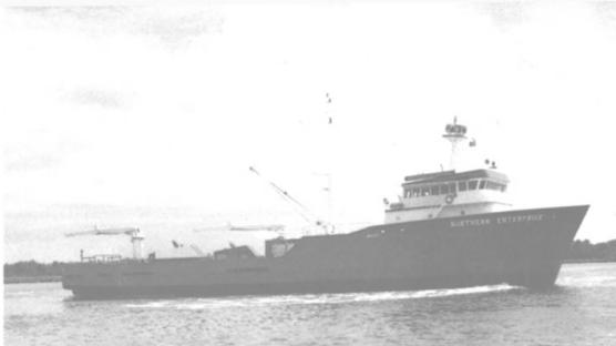
The Northern Enterprise is shown above after conversion. The crabber/processor is powered by two EMD 12-567-BC diesels with Falk 2.98:1 reverse/reduction gears.
