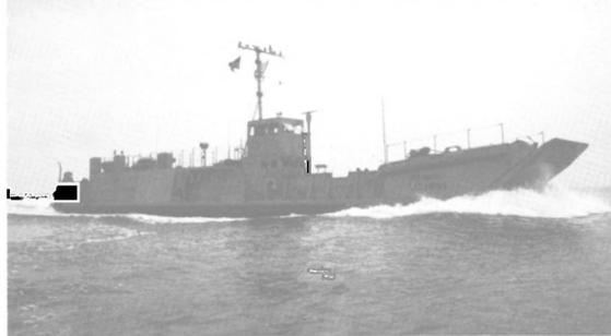
The LCU-1680, powered by twin Detroit Diesel 12V71TI engines, was recently delivered by Moss Point Marine, Escatawpa, Miss., to the U.S. Navy.
