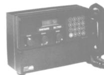
The new RS-7100 VHF radiotelephone. played on a backlighted LCD. Construction is of diecast aluminum and the unit can be mounted on tabletop, bulkhead, or 19-inch rack. Remote stations are extremely compact and have control panels identical to the master station. All sta-
