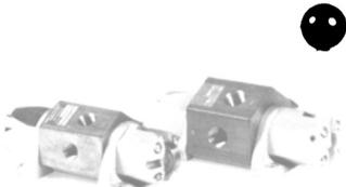
For hydraulic & pneumatic system control—2, 3 or 4 way operation—lapped stainless steel spool & brass body. Direct ported or manifold mount. single or stacking actuators. mechanical. direct solenoid. solenoid pilot & direct pilot—1 8" to 1 2" ports—NPT or SAE—hydraulic service to 2000 PSI—pneumatic to 150 PSI—Catalog AA-300
