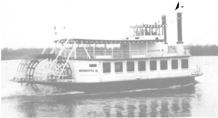
The Cummins-powered Henrietta II is estimated to have a fuel consumption of only 3-4 gallons an hour per engine.
