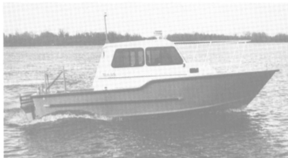
MonArk 28-foot "Protector" achieved 48 mph powered by twin 225-hp Yamaha V-6 outboards.
