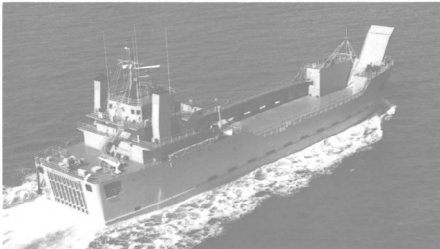
The CW3 Harold C. Clinger, the second in a series of four landing support vessels being built by Moss Point Marine for the U.S. Army, is propelled by two GM-EMD 16-1645-E2 diesel engines.
