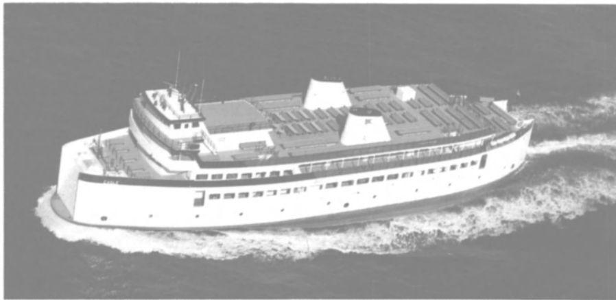
The Eagle, built by McDermott Shipyard, New Orleans, La., is powered by two GM 1,500-hp diesel engines.
