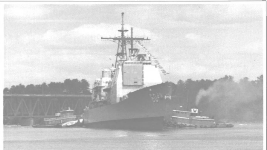
Powered by four GE LM2500 gas turbine engines, the USS Normandy (CG-60) is the third Aegis cruiser built by Bath Iron Works.
