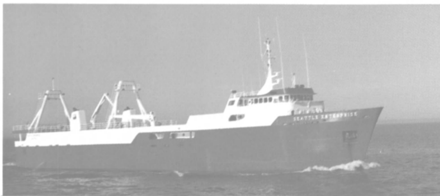
The EMD-diesel-powered Seattle Express is capable of transforming fish into low-cholesterol fish paste (surimi), used to make imitation crab meat, shrimp and other products.
