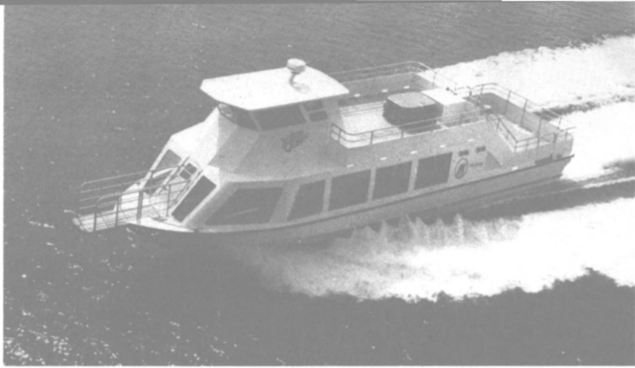
The Munson Manufacturing-built Yukon Queen is powered by Triple Lugger's L6140A engines coupled to three Hamilton waterjets.
