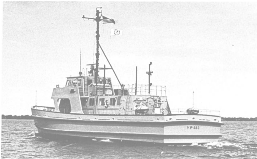
The YPs are of wood hull construction, with an aluminum superstructure, overall length of 108 feet, beam of 22 feet 9 inches.
