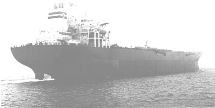
The Fredholm is powered by a single five-cylinder, two-stroke MAN B&W L70MCE engine, which develops 10,900 bhp.
