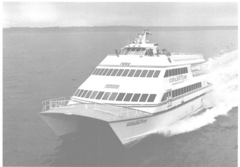
The Catalina Flyer, built by Nichols Brothers Boat Builders, Whidbey Island, Wash., is powered by two specially lightened Caterpillar 3516TA diesel engines.
