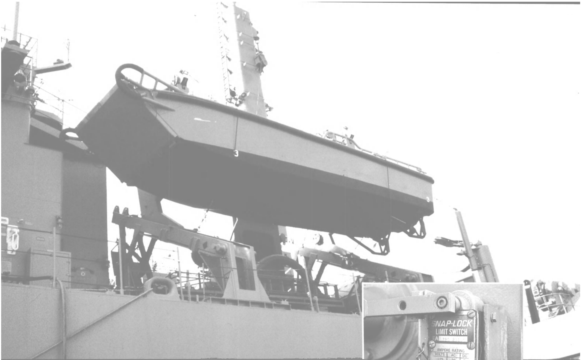
Mechanical limit switches are still preferable to electronic proximity switches in most Navy applications. Here, a Namco Snap-Lock® switch controls a davit gearbox. Rugged Snap-Lock switches have reliably stood up to harsh environments like this for years.
