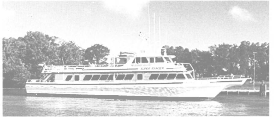
The Super Ranger, built by Gulf Craft, Inc., is powered by three Detroit Diesel engines, which produce a total of 2,160 shp at 2,300 rpm.
