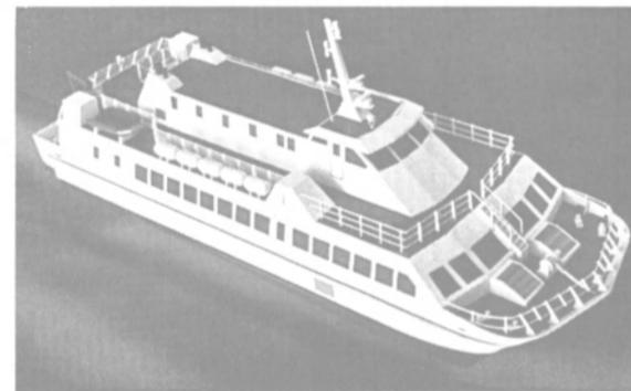
Model of the SES-Jetrider vessel. Two of this type of ship are being constructed in Sweden for use as high-speed passenger ferries.
