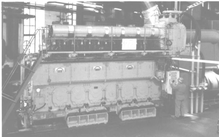
The diesel engine type shown, MAN B&W Diesel's 6L 40/54, will be used as part of a four-engine "father-and-son" power plant aboard a new Chandris cruise ship being built by Meyer Werft, Papenburg.
