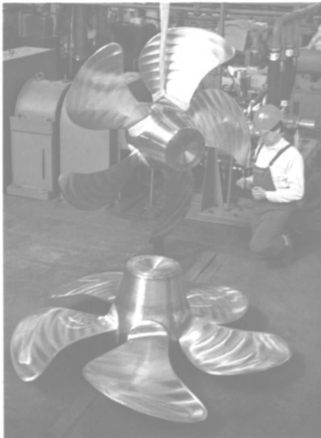
Nonmagnetic C.P. propellers for a mine countermeasure vessel.
