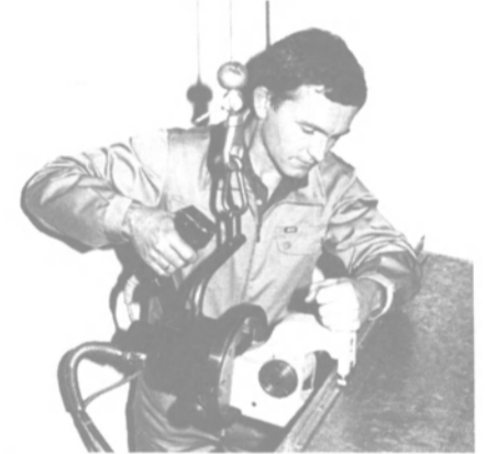
The photo shows an Eckold mobile tool for press-joining air ducts.
