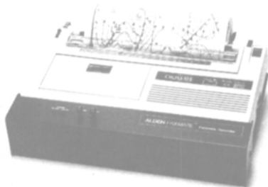
The low-cost Alden Faxmate Weather Chart Recorder doubles as a printer for onboard computer.
