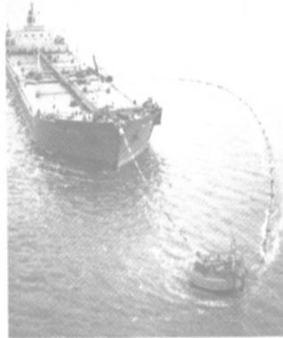
Single Point Mooring (SPM) systems designed for ropes made with Spectra high performance fibers from Allied-Signal Inc., offers extremely low water absorption, the highest resistance to the toughest abuse, as well as neutral buoyancy—it floats. Photo courtesy of Samson Ocean Systems, Inc.
