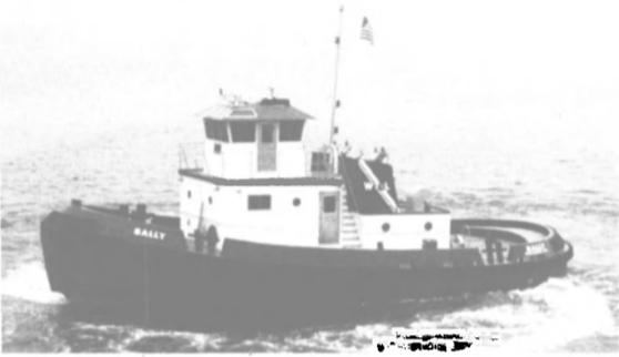
The twin-screw, 360°-rotating-nozzle, ship-docking tug Sally is powered by two G.M. Detroit Diesel Allison engines rated 900 shp at 2,400.
