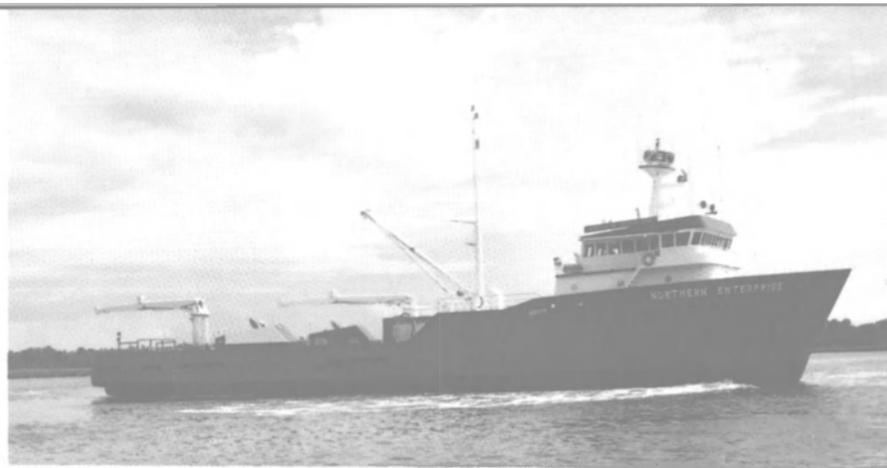
marine engines coupled to Nomera 12 jet pumps, she can reach speeds in excess of 25 knots. The jets have diverter and check valves engineered by North American Marine Jet, Inc., to divert water flow into the firemain system.
