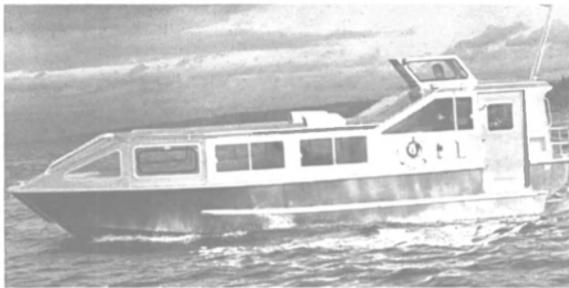
Fully enclosed and capable of high speed with a flat wake, the HST Reliable was specially designed for operation in harbors.
