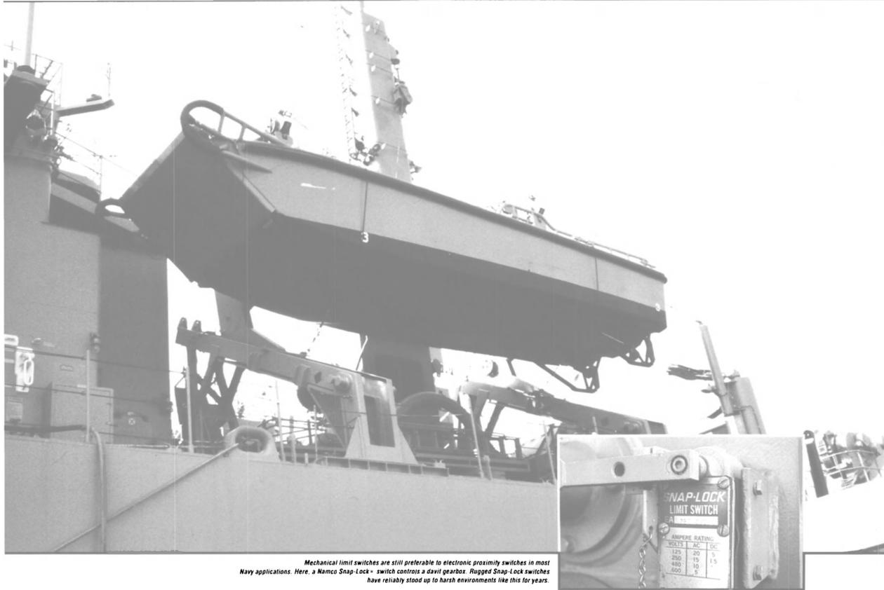
Mechanical limit switches are still preferable to electronic proximity switches in most Navy applications. Here, a Namco Snap-Lock™ switch controls a davit gearbox. Rugged Snap-Lock switches have reliably stood up to harsh environments like this for years.
