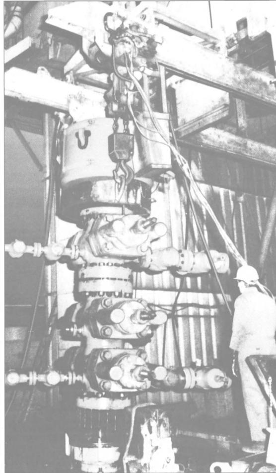
They are for instance standard built for application in areas where there is a risk of explosion. Explosion proof requirements are especially high on drill platforms. For this reason increased sparking protection is possible as an optional extra. JDN-pneumatic hoists are available with carrying capacities from 0,1 to 100 tons.
