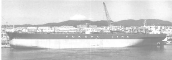
Heavy Industries Co. Ltd. (HHI) in Korea delivered the 254,000-dwt Very Large Crude Carrier (VLCC) Yukong Frontier to her owner, Yukong Line Ltd. The ship is the standard type developed by Hyundai Shipyard, and the first in a series of three VLCCs ordered for Yukong Line.
