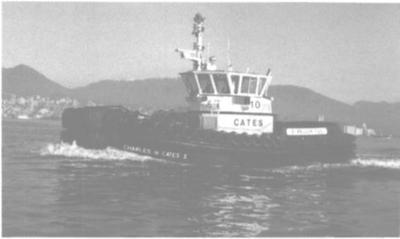
The ship-handling tug Charles H. Cates X features a hull of all-welded steel, double-chime form, with transverse framing, which is unique to the Cates fleet. The hull form was developed jointly by the company and naval architect Robert Allan Ltd.
