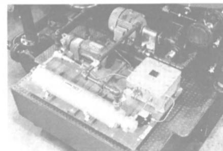
Shown is a Kim Hotstart prelube/postlube system in an industrial engine application. The system keeps critical engine parts cool or warm and prevents engine wear.
