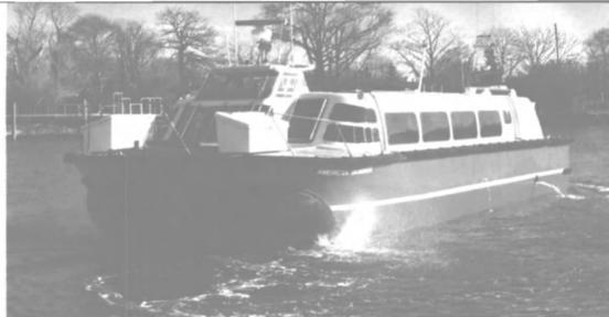
The American Skimmer operates in commuter service between Glen Cove, Long Island, and Manhattan. The hover ferry, powered by Cummins marine engines, is able to make her commuter run in 55 minutes.
