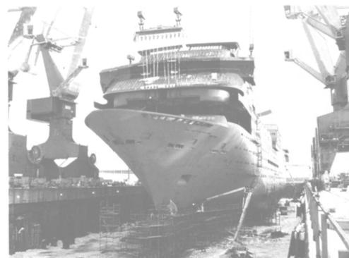
The Fantasy, one of three 70,000-grt cruise ships being built for Carnival Cruise Lines, under construction at Wartsila Marine's Turku shipyard.
