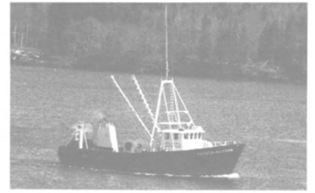
The 70-foot-long Theresa & Allyson is powered by a Caterpillar 3408 DITA with a Twin Disc 516 6:1 reduction gear.
