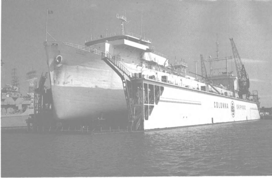
With a 17,200-ton floating drydock (shown above), three marine railways and a full array of ship and pier facilities, Colonna's is able to undertake a wide range of in-plant ship repair jobs for ships up to 800 feet.
