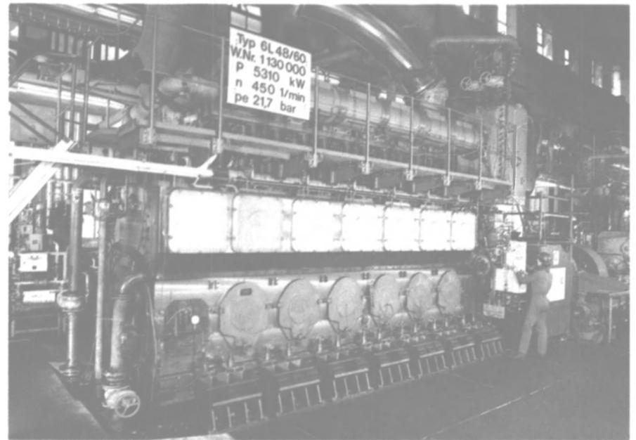
The most recent development in MAN B&W medium-speed four-stroke engines is the L48/60 engine with a cylinder output of 885 kw at 450 rpm. The photograph shows a six-cylinder engine on the test bench in Augsburg Engine Works.
