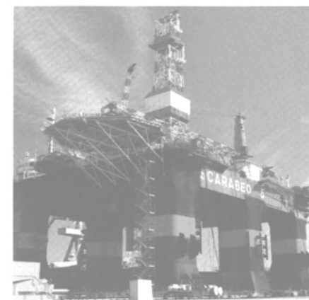
Semisubmersible drilling rig Scarabeo 5, now under construction at the Sestri Ponente shipyard of Fincantieri, will have a drilling capability of up to 7,600-10,000 meters.
