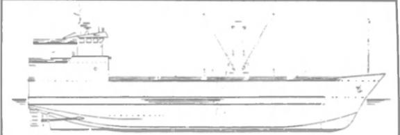
UNDER CONSTRUCTION 195'x41'6"x18' Fish Tender. New, designed for ocean service.
