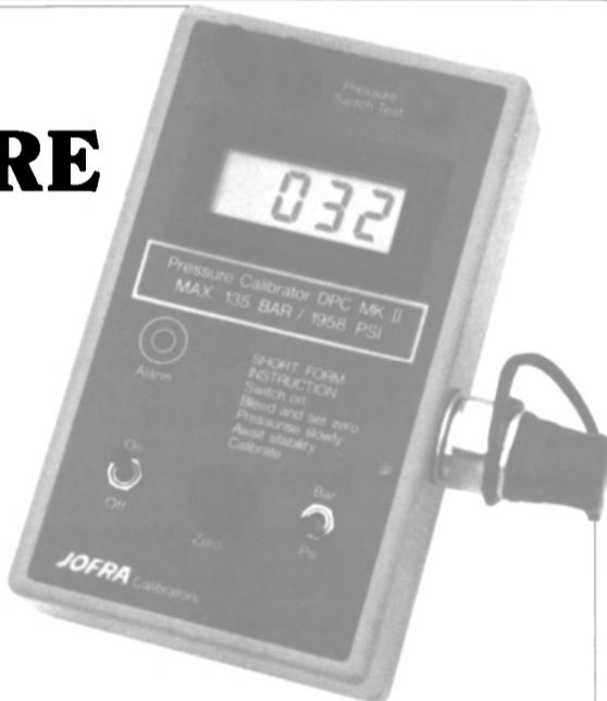
If you need to adjust gauges, pressure switches, transmitters, transducers, safety valves, fuel nozzles or pressure systems you need a Jofra DPC. The DPCs accept hydraulic oil or water as their media and are supplied with a screw pump.
