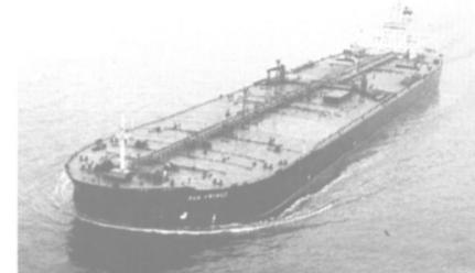
The cargo oil pipes on the Sea Prince are arranged to allow simultaneous storage of three types of crude oil and are coated with high-grade paint to ensure corrosion protection. A stripping system shortens loading time and reduces labor costs.
