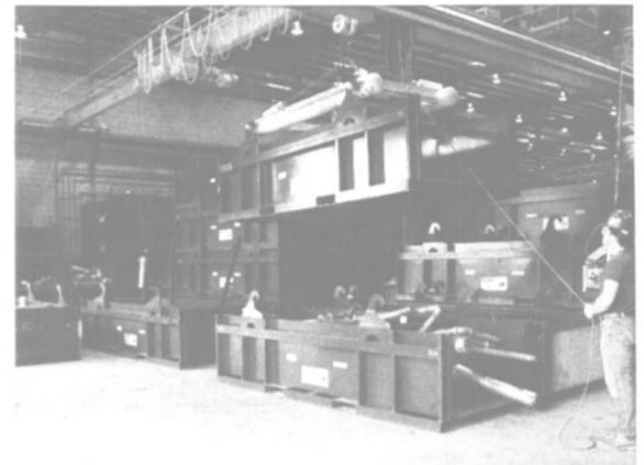
Material handling is simpler and safer at BIW with the new HF Cradle System from Dwight Foote, Inc. The designs of the container and self-aligning and interlocking cradle system create a one-piece unit that can be handled from the floor by one man using an overhead crane and an HF system spreader beam.
