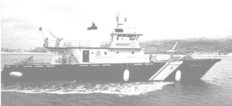
The Moku Ahi is a fully automated firefighting and rescue vessel manned by a crew of five. All engines and firefighting systems can be operated from the pilothouse.
