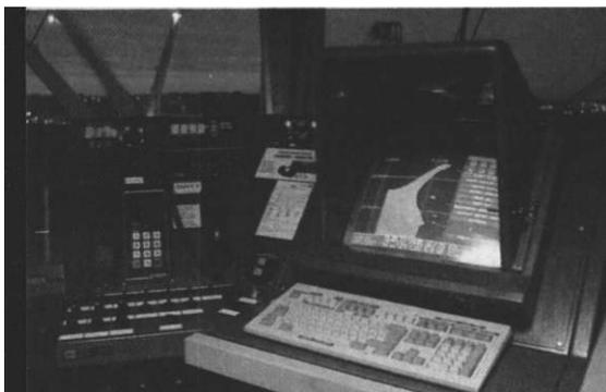
Photo, left: To the right, the voyage management station with the Sperry Marine route control system. To the left, the communication panel.
