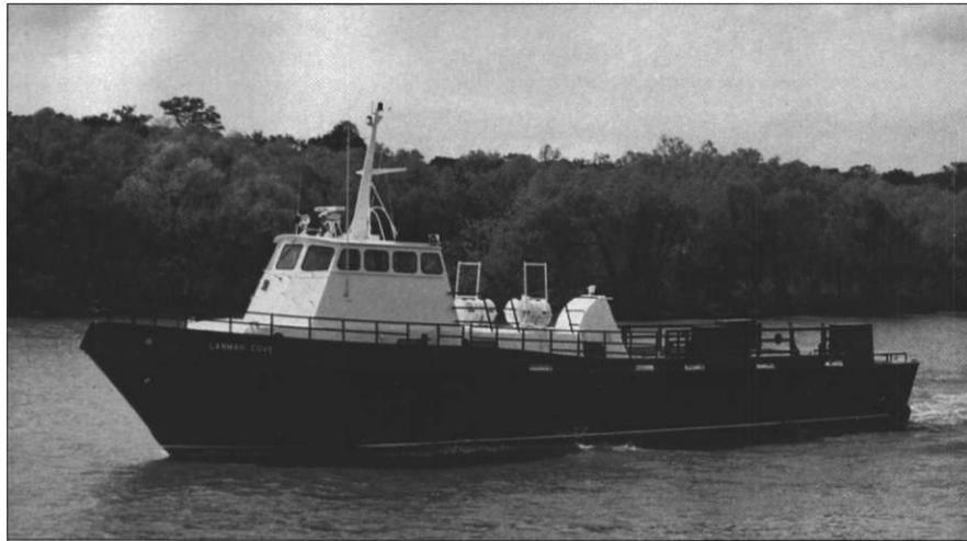
Aluminum Boats' workboat Lanmar Cove has a flush 15-foot by 34-foot aft deck, providing 510 square feet of clear cargo area for a deck load of up to 20 long tons.
