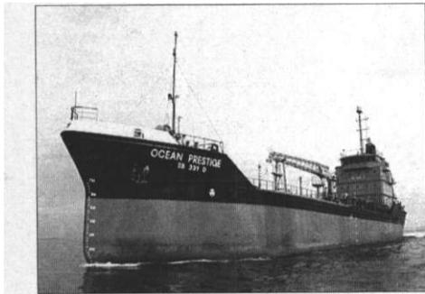
The Ocean Prestige is outfitted and equipped for bunkering and the transportation of cargo oil having flash point above 60 degrees C (140 degrees F). The vessel is steel welded with twin diesel engines and twin fixed-pitch propellers.
