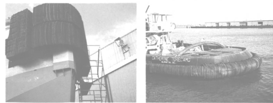
At left, a Viking Fender Company bow fender and, at right, a stern fender. Viking specializes in tug fendering for ship docking, barge handling and submarine handling applications.
