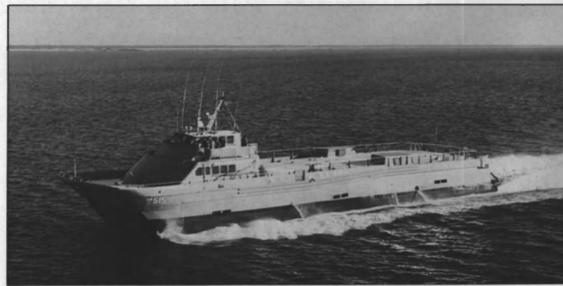
The SES-200, the U.S. Navy's only Surface Effect Ship, is now able to reach speeds in excess of 40 knots, following her conversion, modification and upgrading at Textron Marine Systems' New Orleans shipyard. Her propulsion system now features MTU engines, ZF gearboxes and KaMeWa waterjets.
