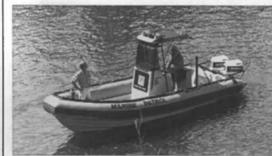
The self-righting system of Zodiac/Hurricane's RHI will enable the vessel to negotiate heavy surf and sea conditions.
