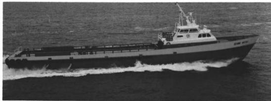
The 160-foot crewboat Deanne McCall is powered by six Cummins diesel engines to a speed of 24 knots.
