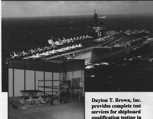
Dayton T. Brown, Inc. provides complete test services for shipboard qualification testing in accordance with MIL-S-901 Shock, MIL-STD-167 Vibration, and MIL-E-16400 test requirements.
