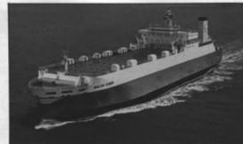
The Baltic Eider, a modern RO/RO vessel built in Korea for UBS, London. She and her sister vessel have a father-and-son arrangement with one six-cylinder and one eight-cylinder Wartsila Vasa 46 engine.
