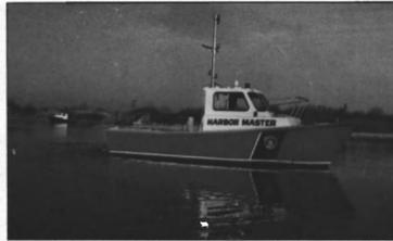
The new 7.4 meter Harbor Master can be powered by outboard, inboard/outboard and jet drive propulsion systems.
