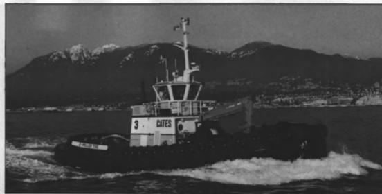
One of the unique features of the Cates 3 is the line-handling crane on the foredeck. An Atlas extending, knuckle boom crane is used to transfer the tug's nylon/polyester hawser to the deck of an attended ship.
