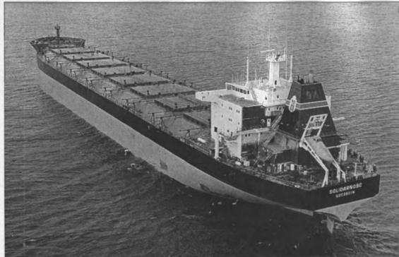
The bulk carrier Solidarnosc, recently delivered by B&W, features a new bow form which offers larger cargo volume and easier access to Hold No. 1, while maintaining the same performance standard.
