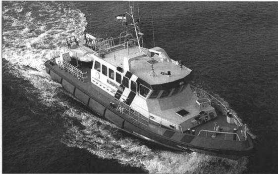
The police surveillance launch RP 9, built by Damen Shipyards, is capable of coming alongside ships with a dangerous cargo in accordance with ADNOR appendix B (requirements valid for tankers).
