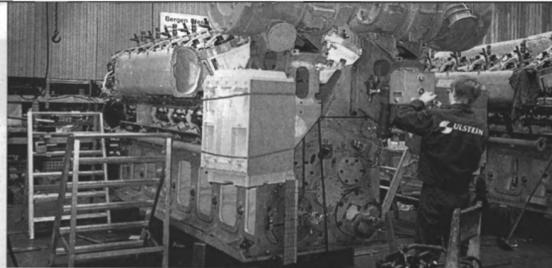
Bergen Diesel in production at Bergen's diesel engine plant in Bergen, Norway. The engine is destined for a Kloster Cruise ship.
