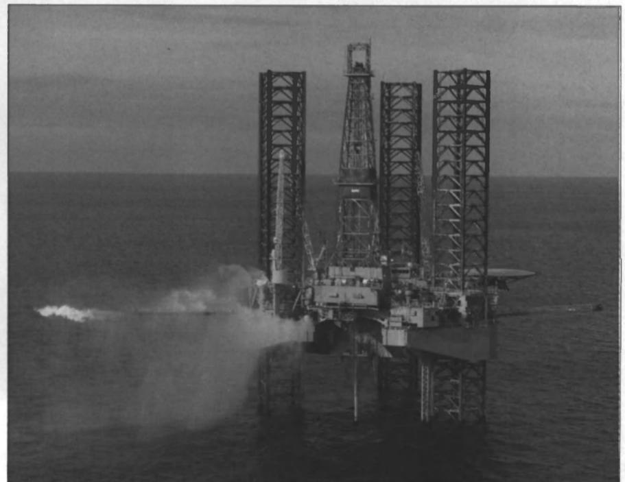
Natural gas is flared from the ODECO jack-up rig Ocean Titan during production testing of a confirmation well in the Gulf of Mexico.
