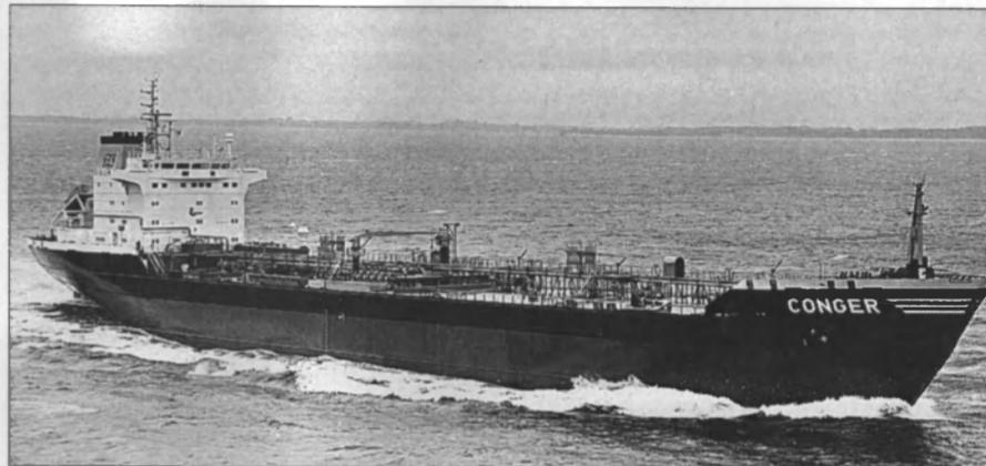
The transportation of five different, fully segregated cargoes is possible at the same time on the chemical tanker Conger, recently delivered by Lindenau.
