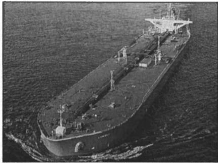
Designed to carry 2 million barrels of cargo oil and cruise with minimal resistance and fuel saving, the 1,076-foot-long by 187-foot-wide tanker Sawako has a new simplified hull structure that eliminates the center girder.
