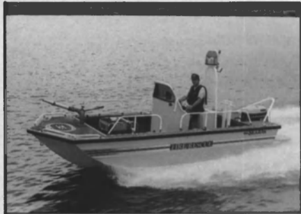
The 19-foot all-aluminum fireboat delivered to the Grapevine Fire Department in Texas.
