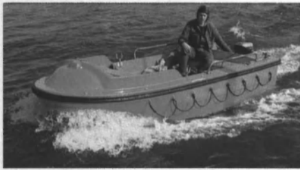
Fassmer's 13.7-foot rigid rescue boat is equipped with a gasoline-driven outboard engine and offers speeds exceeding 6 knots.
