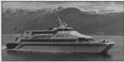
The new Kvaerner Fjellstrand-built high-speed passenger catamaran Springaren can carry a total of 255 passengers, divided between 216 on the main deck and 39 on the upper deck.
