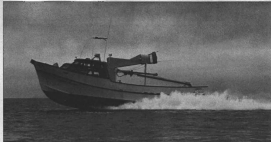
Skipper/owner Ray Wadsworth's 58-foot, 3,000-hp fast fishing boat Order of Magnitude, built by Kodiak Marine Construction of Sequim, Wash. Her fish-spotting tower/mast folds down aft to help her gas turbine engine power her to over 50 knots.
