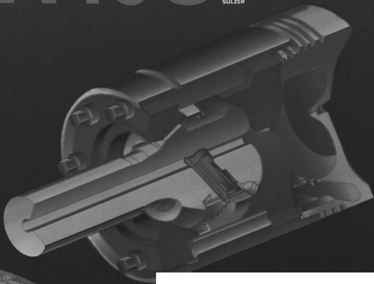
Rotating pistons bring the same benefits to Sulzer ZA40S engines as does revolving satellites - equalizing temperatures and thermal loads.
