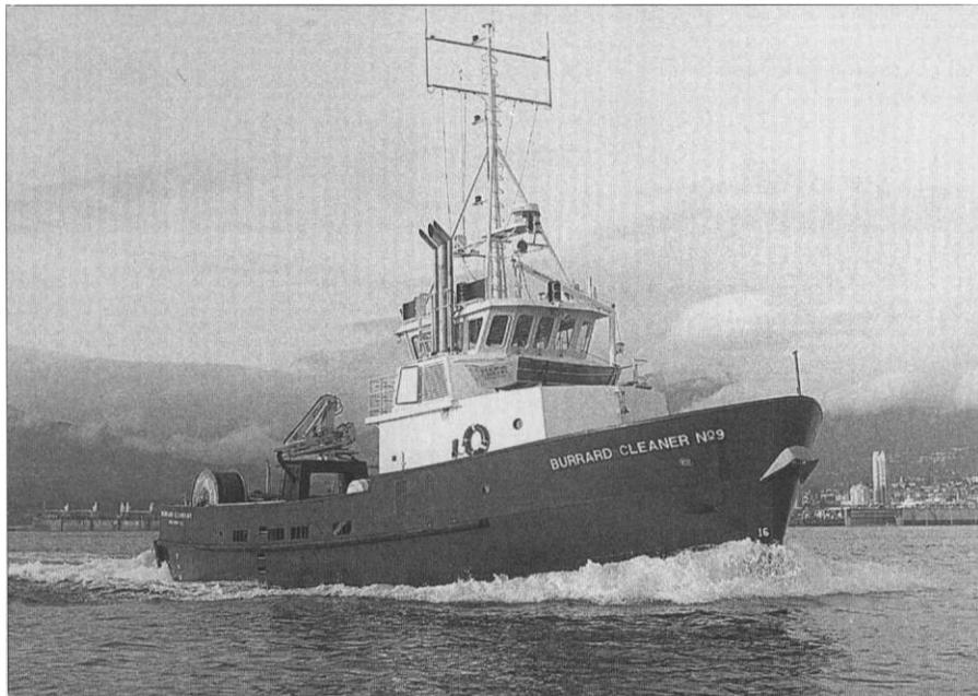
The 75-foot Burrard Cleaner No. 9, designed by MARCO Pollution Control of Seattle, is the largest oil spill recovery vessel serving Canada.
