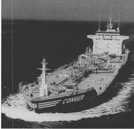
The MAN B&W-powered Conger has specially developed ship lines for an optimized speed/power characteristic and good seakeeping properties. Her Jastram-Werke bow thruster improves maneuverability, while her double bottom and double side shell lower the risk of environmental pollution.
