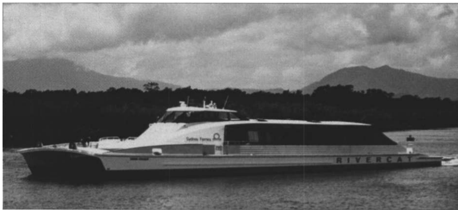
The aluminum-hulled Rivercat, first of seven catamarans for the State Transit Authority, Sydney, is propelled to over 23 knots by a pair of Schottel Rudderpropellers.
