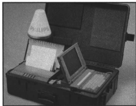
Philips Safecom CP. Standard 'C' Inmarsat portable terminal in a self-contained suitcase.
