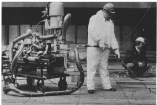
BoatLIFE's 2 Part Polysulfide Meter, Mix, and Dispensing Unit is used here to lay in the sealant. No need to mix and pour into caulking guns—saving time and money!
