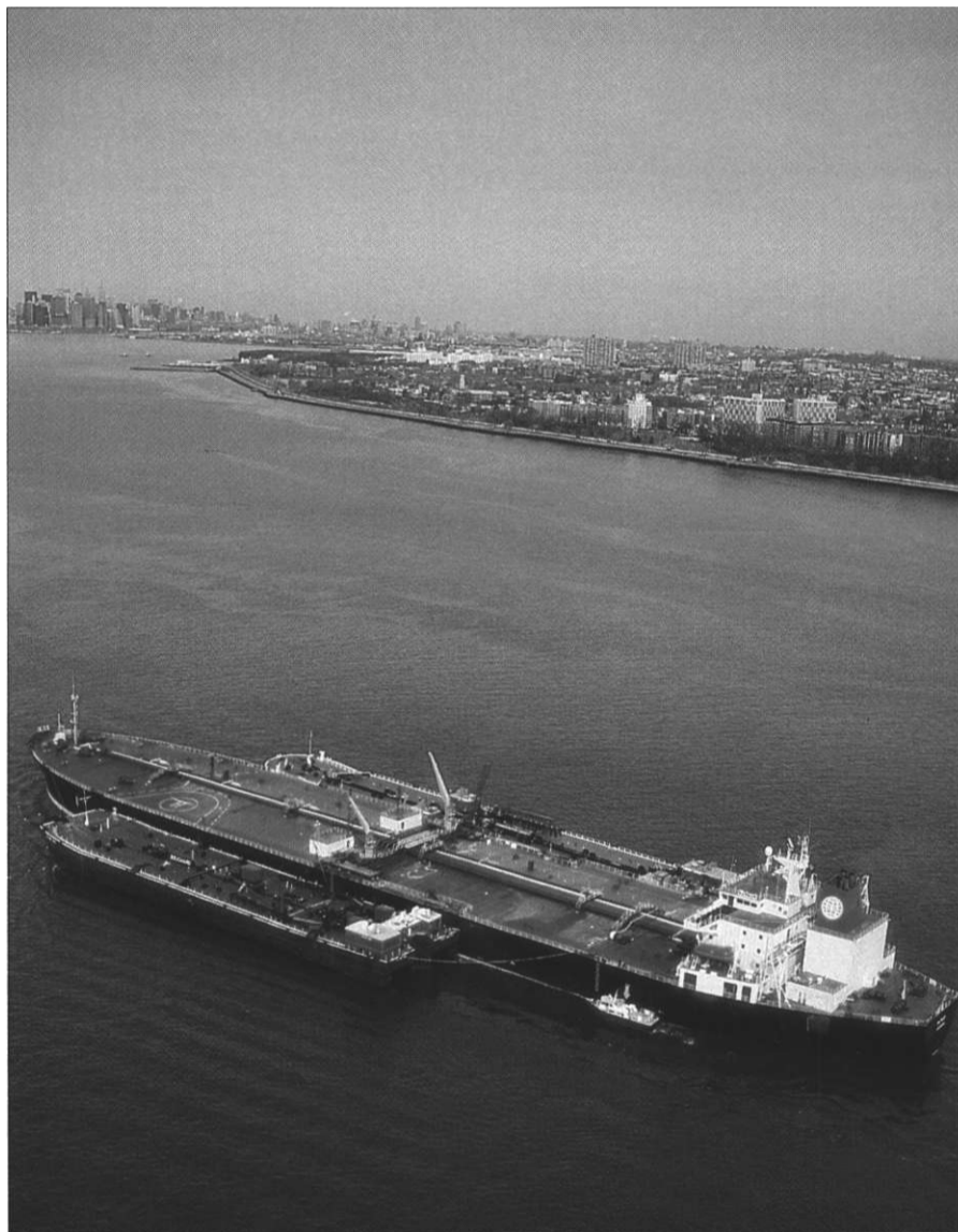
The recently delivered double-hulled crude tanker Patriot on her first cargo trip to New York. She is the first of four 95,000-dwt tankers being built by Samsung Heavy Industries of South Korea for Conoco Shipping of Houston.
