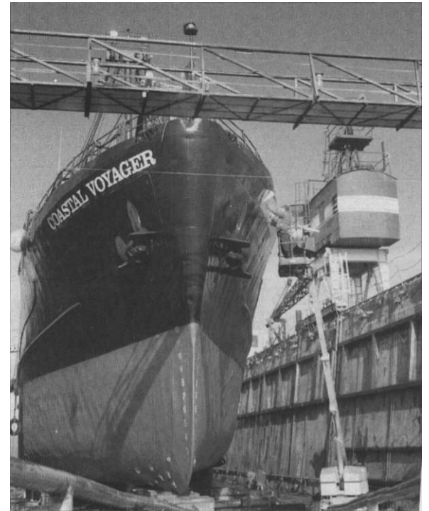
The freighter Coastal Voyager receiving paint and steel work in Marine Industries Northwest's MINI I drydock.
