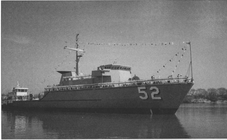
The USS Heron (MHC-52), second of a new class of GRP-hulled U.S. Navy minehunters built by Intermarine USA, Savannah, Ga.
