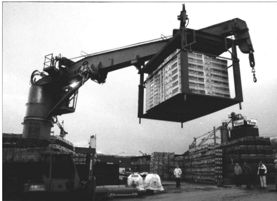
The Pallet Swinger, the latest development from Hagglunds, has been installed on a number of new reefer vessels.
