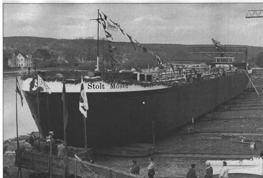
The M/T Stolt Mosel, built by Bayerische Schiffbau GmbH shipyard in Erlenbach, Germany, is one of five 2,100-dwt inland chemical tankers designed by Stolt-Nielsen to transport bulk liquid along the Rhine.
