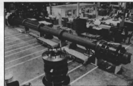
IMO Pump's vertical deep-well screw pump.
