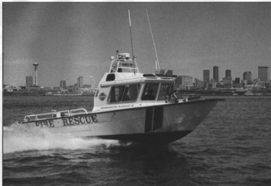
This fire, search and rescue boat from Workboat Northwest features a Kodiak gasoline engine and Berkeley pumps.
