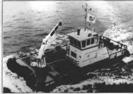
An 88.2-ton Effer marine crane operating from a Dutch work boat.
