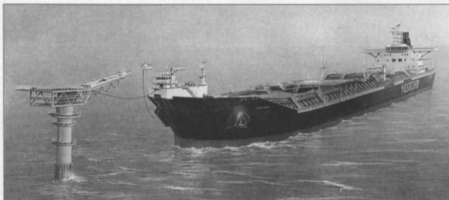
An artist's drawing of a Futura class tanker fitted with a bow cargo loading station.
