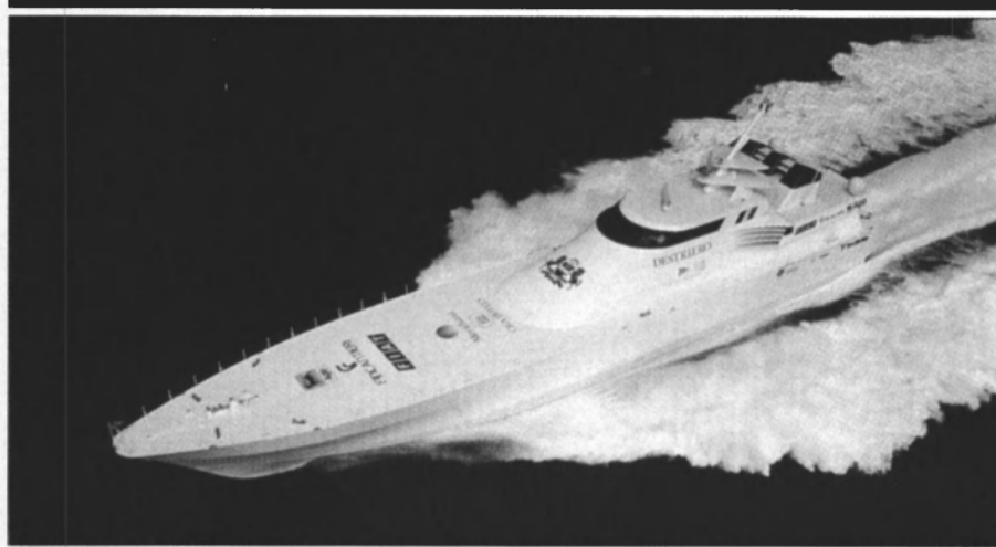
Three LM1600 gas turbines power the Italian high-speed vessel, Destriero, which has a speed capability of more than 60 knots.
