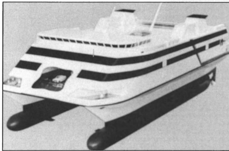
This 250 car, 876 passenger ferry from Swath Ocean can attain 36.5 knots.
