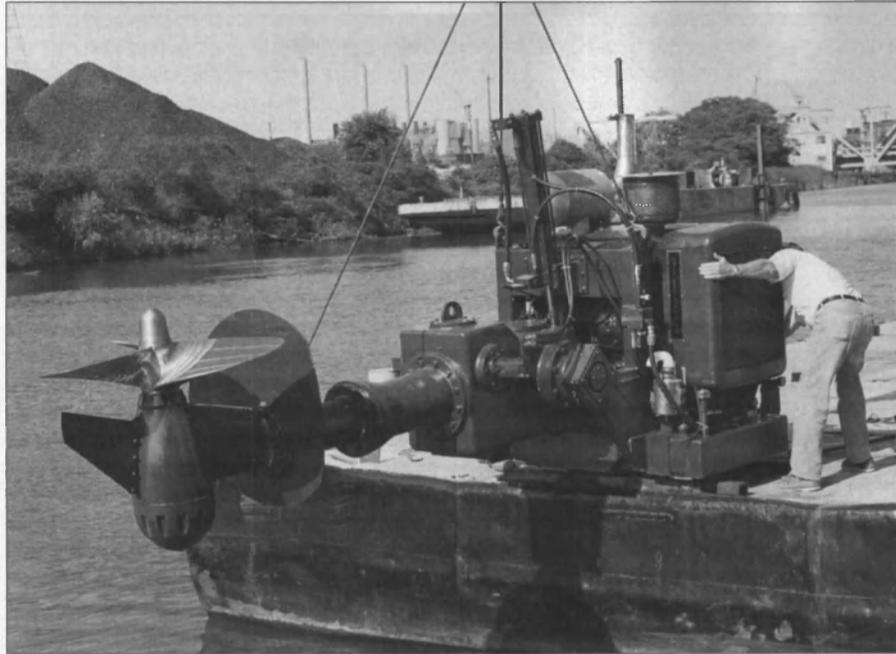
Harbormaster SW3150 being positioned onboard a 40-foot barge
