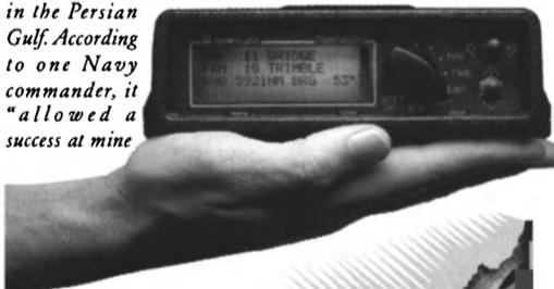
**Ultimate Accuracy.** For ultra-precise navigation, a technique called "Differential GPS" can give you 2-5 meter accuracy. Soon coastlines will be dotted with radio beacons like the one at Montauk N.Y., broadcasting corrections to GPS receivers in the area. Only Trimble products come standard with the ability to accept these corrections.
