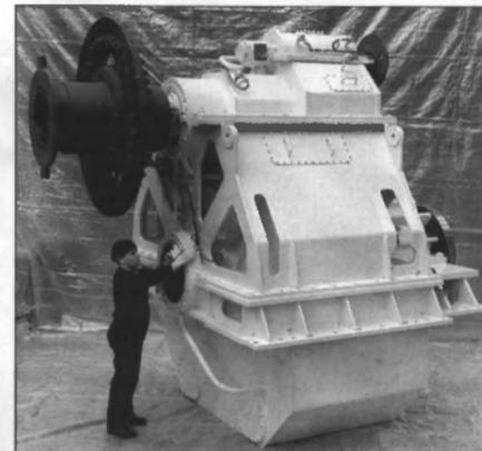
One of the reduction gears being built by Schelde Gears Vlissingen for two containerships.
