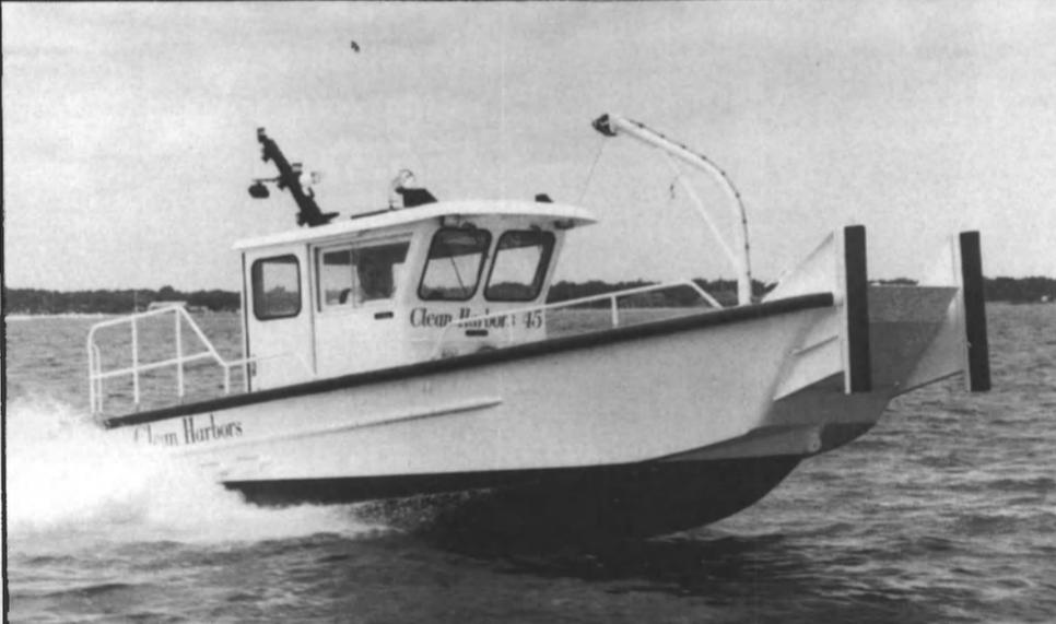
The 30' Oil Clean Up Boat engineered and designed for effective spill control. Powered with twin diesel engines and heavy duty aluminum construction, it offers a quality solution derived from over 32 years of service to the maritime industry.
