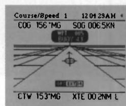
**Measure performance.** GPS can measure your speed over the ground to a tenth of a knot, so you can precisely figure the set and drift of even subtle currents. That helps you stay on course and helps you find optimum engine and rudder settings.
