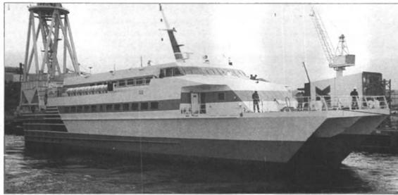
The 300-passenger Han Ma Eum Ho catamaran passenger ferry is powered by Paxman Diesel 18CM engines.
