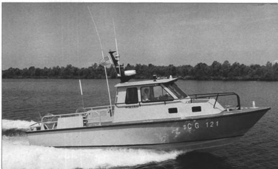
SeaArk's new Dauntless vessel is a deep vee hull design.
