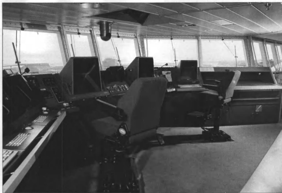
A typical Sperry Marine Voyage Management System (VMS) integrated navigation and control system.
