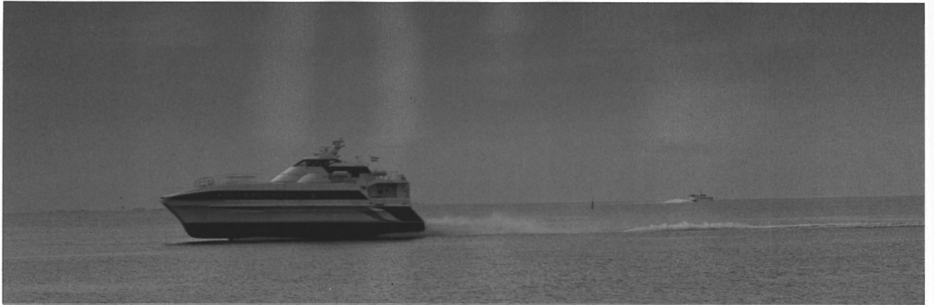
Westamarin's Foilcat 2900, driven by two MTU 16V engines, is capable of 50-knot speeds.
