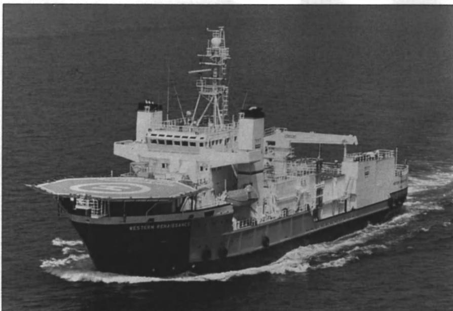
The Western Renaissance, reportedly the world's largest and most advanced well stimulation vessel, was christened by The Western Company of North America. The 308-foot ship was designed and built to provide proppant fracturing, acid fracturing, matrix acidizing and nitrogen services in the North Sea.
