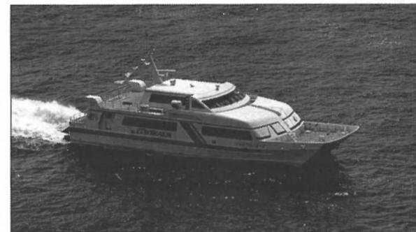
The Trident Ace, first of Hitachi Zosen's Superjet-30 series of foil-assisted catamarans.
