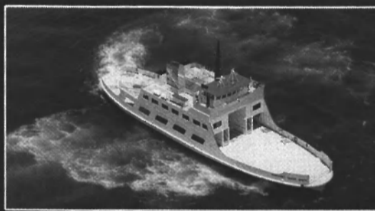
MARGARET CHASE SMITH - 166' x 40' double ended ferry boat with a capacity of 226 passengers and 30 autos built for the State of Maine, for transportation between Isleboro and Lincolnville, Maine.
