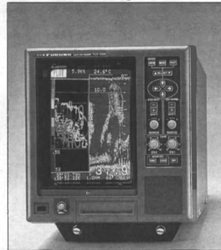
Furuno's new FCV-1000 sounder displays 16 colors or multiple levels of amber.
