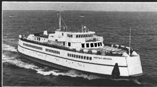
MARTHA'S VINEYARD - 230' x 60' passenger/vehicle ferry operating between Woods Hole and Martha's Vineyard. The double-ended ferry was built for Woods Hole, Martha's Vineyard and Nantucket Steamship Authority and has the capacity to transport 1387 passengers, 17 crew members and 70 vehicles.
