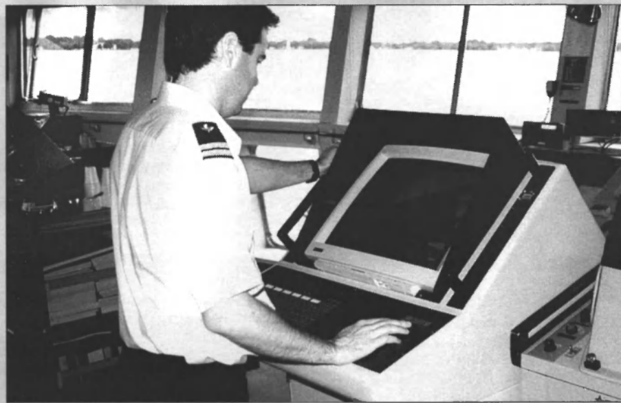
ECDIS systems integrate sensor data into an electronic chart display.
