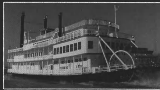
DIAMOND LADY - 201' x 46' Sternwheel Casino Vessel built for Steamboat River Cruise Lines, Bettendorf, Iowa. This 1200 passenger casino vessel.
