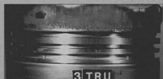
Fig. 3: The condition of the piston after more than 500 running hours on heavy fuel oil. Note the clear ring grooves and piston lands.
