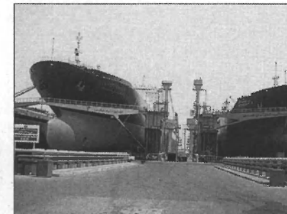
Vessels in ASRY's floating docks, which can accommodate ships up to 120,000-dwt.
