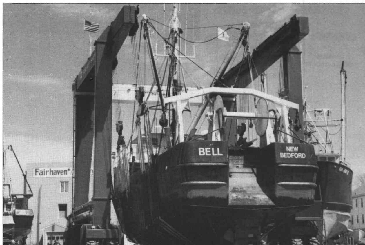
A model 300 BFM mobile hoist at Fairhaven Shipyard, Fairhaven, MA.
