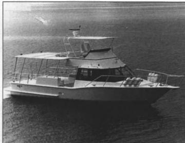
Munson Manufacturing of Edmonds, Wash. completed a 45-ft. (14-m) dive boat for a customer in Saudi Arabia. Designed to operate at speeds in excess of 46 knots, its deep-vee hull
