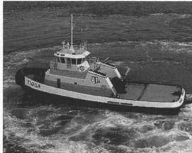
Tri-Star Marine of Seattle has delivered a 4,000 hp tractor tug, *Tioga*, to Coos Bay Towboat Co. of Oregon. The new 85-ft. (26-m), ice-strengthened boat was designed and built by Tri-Star, with engineering services provided by Jensen Maritime Consultants.
