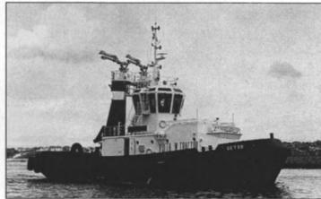
Astilleros Zamacona, member of the Construnaves group of shipyards, made the first two deliveries of an order for four multi-purpose Voith tractor tugs to Spanish towage company Cia. de Remolcadores Ibaizabal. These super-tugs are fitted with Voith-Schneider water tractors driven by two 1,930-bhp Wartsila Diesel engines.
