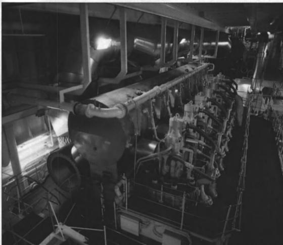
HDW says this slow-speed, two-stroke diesel, Mitsubishi 7UEC85 LSC engine plant installed on its *N. Fribourg* open-top containership driving a fixed-pitch propeller is economical, reliable and easy to maintain. The engine has a nominal output of 27,290 kW (37,100 hp) with 102 min<sup>-1</sup> rpm and a low specific consumption of 165 g/kWh (121 h/tp).
