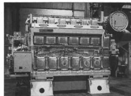
Wartsila Vasa 6R32. This model, as well as a Wartsila SACM Diesel JUD25 auxiliary engine (see pg. 46), was recently installed on seven tankers under construction in the South East Asia region.
