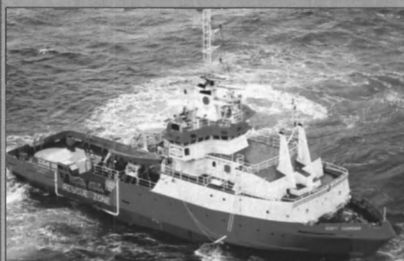
The standby/rescue vessel Scott Guardian , equipped with an Aquamaster propulsion system, is 180 feet (55 m) long with a breadth of 43 ft. (13 m) and depth of 18 ft. (5.5 m).
