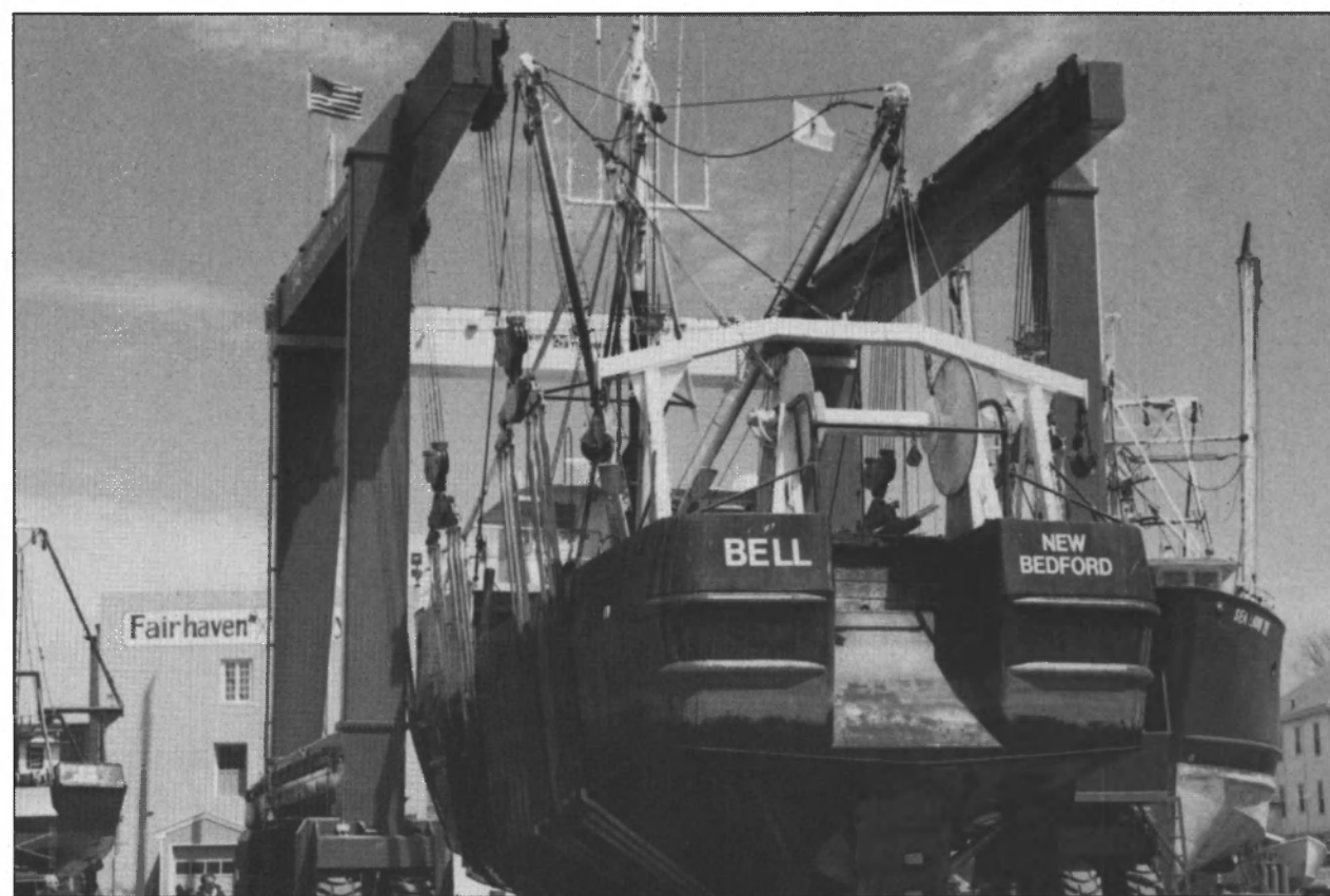
A model 300 BFM mobile hoist rated at 660,000 lbs. shown at Fairhaven Shipyard, Fairhaven, MA.
