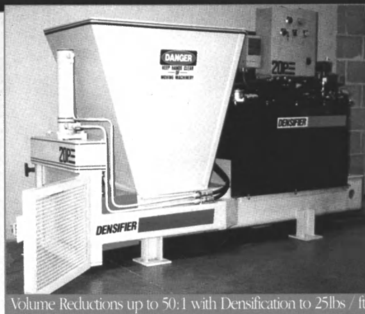
Volume Reductions up to 50:1 with Densification to 25lbs / ft.
