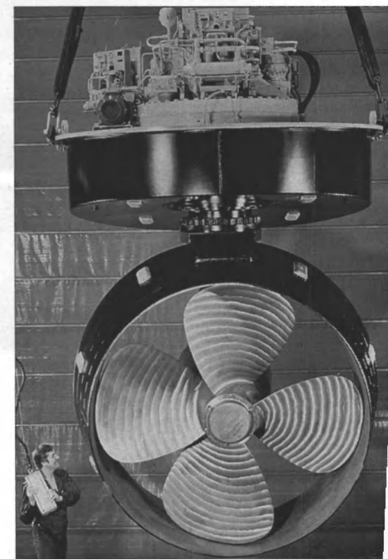
According to Aquamaster-Rauma, the high bollard pull capable six Z-drives it is supplying for three Bay Transportation tugs make them the most powerful Z-drive tugs of their size in the
