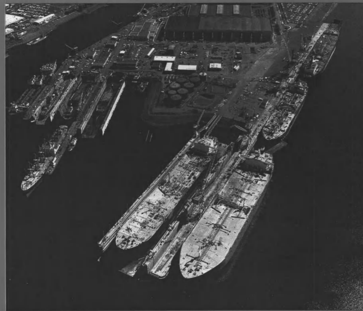
PORTLAND SHIPYARD has three active dry docks, including a 982-ft. x 185-ft. (299.3-m x 56.4-m), 87,000-long ton lift capacity floating dry dock.
