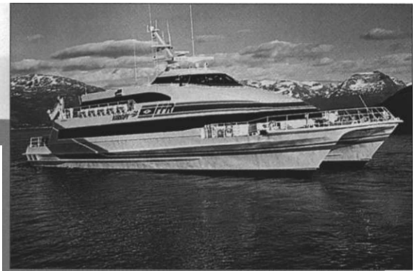
Vessel: ..... Vargoy Type: ..... "Flying Cat" catamaran Builder: .....Kvaerner Fjellstrand Owner: .....Finnmark Fylkesrederi Engines: .....MTU Waterjets: .....Kvaerner Energy
