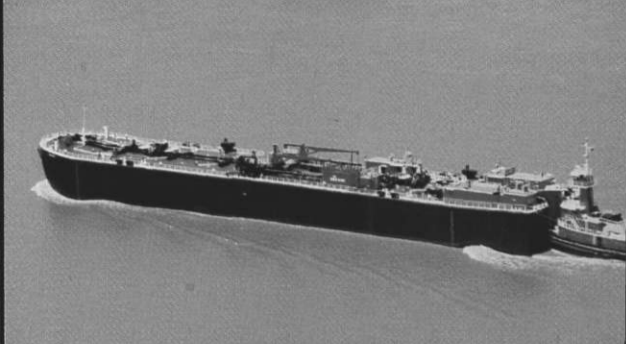
467 Foot Double Hull Tank Barge/127 Foot Tug
