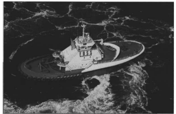
Vessel: ..... Garth Foss Type: .....Tractor tug Builder: .....Trinity Owner: .....Foss Maritime Main engines: .....EMD Propulsion: .....Voith-Schneider cycloidal
