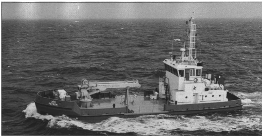
The Kuwait Oil Company says the Effer crane was chosen for its compactness and flexibility, which suited the relatively small Fateen .
