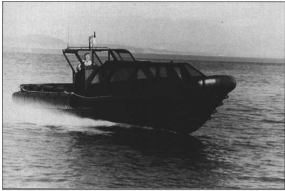
Vessel: .....Team One GB36 RIB Type: .....Assault RIB Builder: ..... American Eagle Mfg. Engines: .....Caterpillar Waterjets: .....North American Marine Jet
