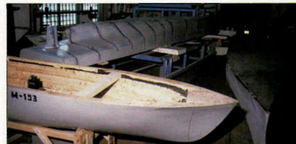
The Institute's model shop constructs wood and/or paraffin wax models for use in its test facilities.
