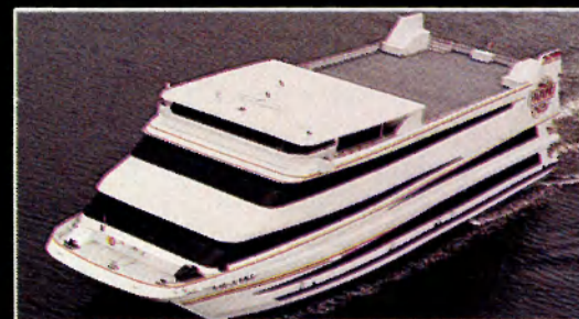
PAR-A-DICE - 240' x 66' triple deck casino vessel built for Par-A-Dice Gaming Corp., East Peoria, Illinois. This ultra modern catamaran style vessel has a capacity for 1,600 persons and 33,000 sq. ft. of casino space.
