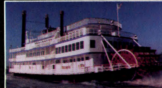
DIAMOND LADY - 201' x 46' Sternwheel Casino Vessel built for Steamboat River Cruise Lines, Bettendorf, Iowa.
