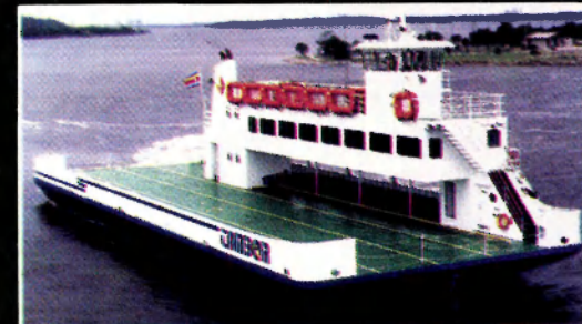
TAMBOR - 130' x 45' double ended passenger/vehicle ferry. The Tambor has a capacity of 375 passengers and 16-24 vehicles.
