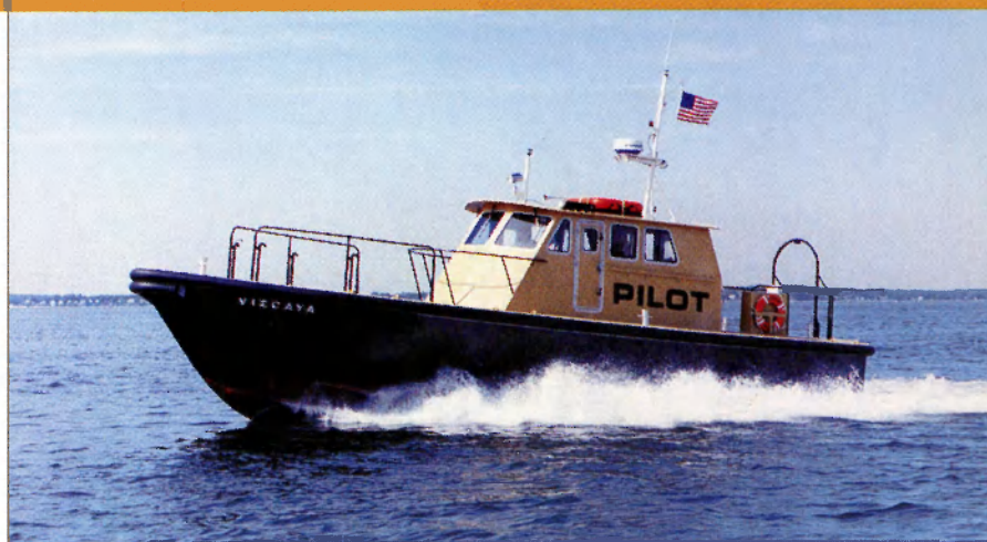
The Vizcaya , a 52-ft. (16-m) all-aluminum pilot boat built by Gladding-Hearn for the Biscayne Bay Pilots Assoc., is powered by Detroit Diesel engines.
