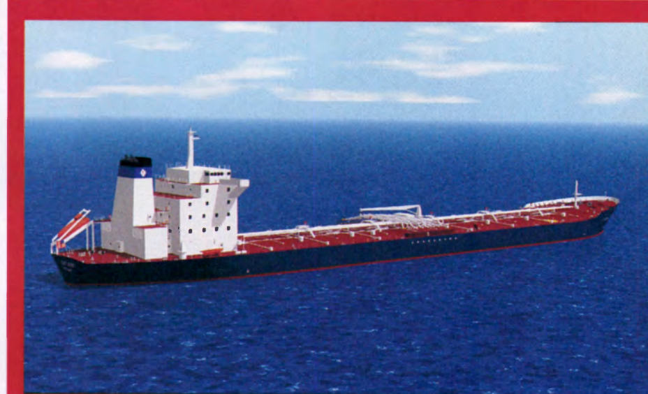
GULF ISLAND TANKER DESIGN FROM INGALLS: This is a computer-generated concept of Ingalls' new Gulf Island Tanker. Designed in-house, Ingalls said this new class of 42,000 dwt product carriers will economically carry petroleum products, meeting all U.S. and international environmental and safety standards. Ingalls also said the Gulf Island design is environmentally sensitive — with a double hull and state of the art navigational and safety features — and economical to operate over the long term, with standardized machinery components.
