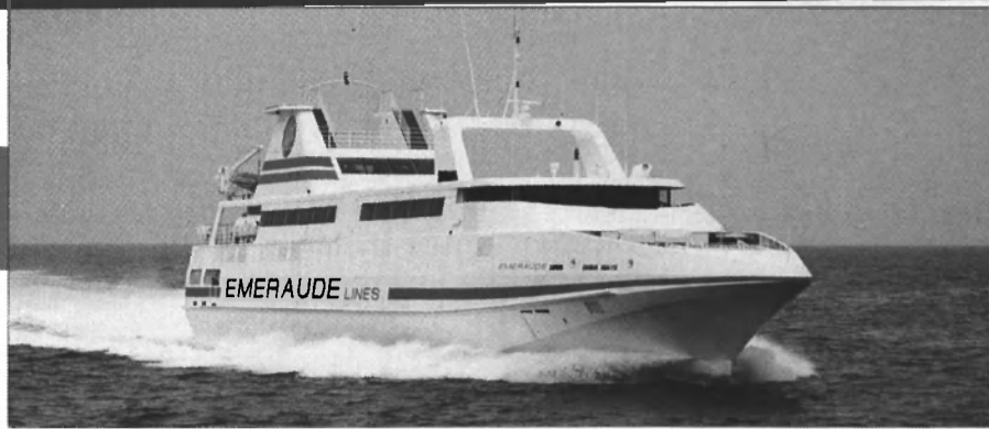
Classed with Bureau Veritas, the Corsaire 6000 fast passenger/car ferry Emeraude entered service between St. Malo and Jersey in May 1994. Built at Leroux & Lotz, the deep-V monohull is built completely of light aluminum alloy and has a top speed of 34 knots.
