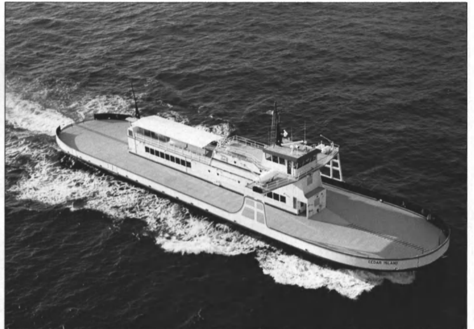
The Cedar Island is a new 300-passenger, 50-vehicle ferry built by Trinity Marine Group's Moss Point Marine for the North Carolina State Department of Transportation, Ferry Division.
