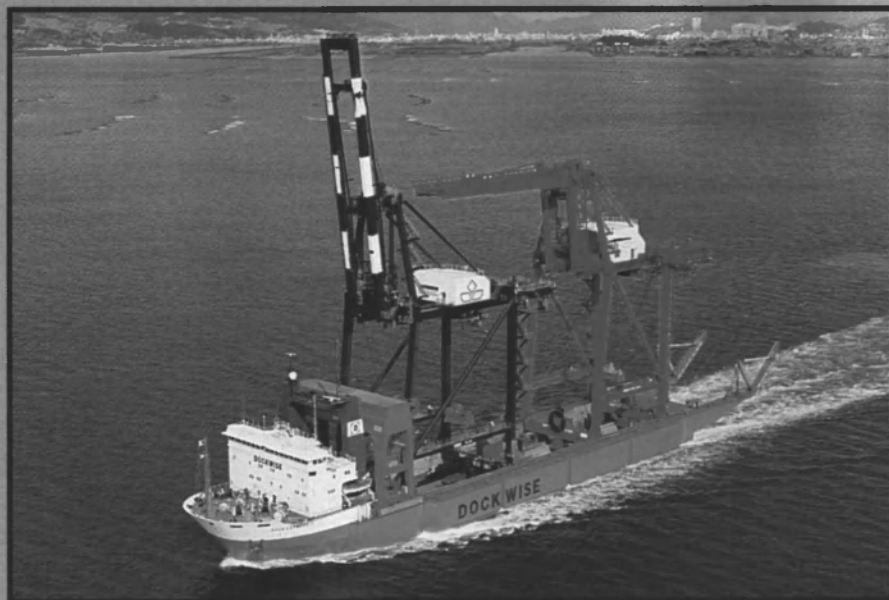
The Dock Express 11 leaving the port of Hiroshima with a cargo of two fully-erected post-Panamax container cranes bound for Hong Kong and Yantian, China, braced with tensioned wires. The red painted gooseneck crane is destined for the MTL Terminal in Hong Kong. The blue painted crane with its boom upright has been delivered to the new terminal in Yantian.
