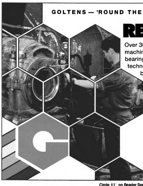
Over 30 years ago, Goltens designed a special machine for centrifugal rebabbitting of bearings. Since then our specially trained technicians have rebabbitted thousands of bearings. We work from original drawings to make sure your bearings are machined to precise tolerances. Downtime is kept to a minimum. So count on Goltens. We'll do the job right away...and we'll do it right.
