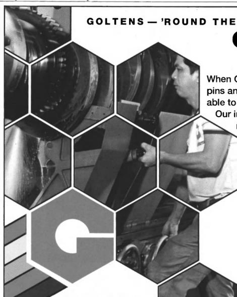
When Goltens reconditions crankshafts, crankpins and main journals, in most instances we are able to do the job without removing the shaft. Our in-situ grinding saves you downtime and money. Or, if your job is best handled in-shop, Goltens has facilities worldwide to do the job fast. And we've been doing it for over 50 years. For all your crankshaft needs, count on Goltens. We'll do the job right away...and we'll do it right.
