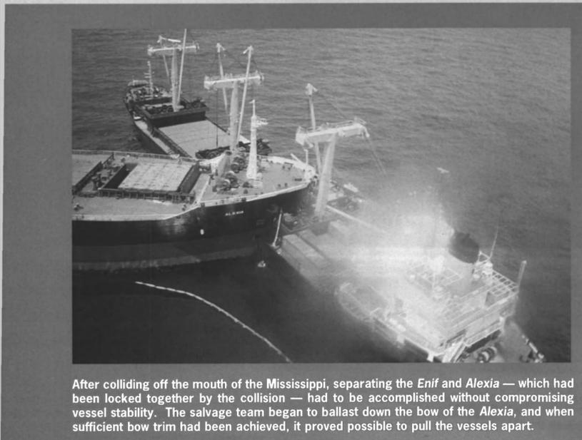
After colliding off the mouth of the Mississippi, separating the *Enif* and *Alexia* — which had been locked together by the collision — had to be accomplished without compromising vessel stability. The salvage team began to ballast down the bow of the *Alexia*, and when sufficient bow trim had been achieved, it proved possible to pull the vessels apart.
