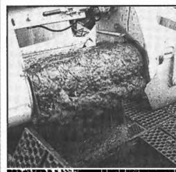
A powerful induction pump behind a Filterbelt system draws heavy oils and debris to a Marco offshore recovery vessel.
