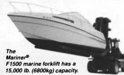
The Mariner® F1500 marine forklift has a 15,000 lb. (6800kg) capacity.
