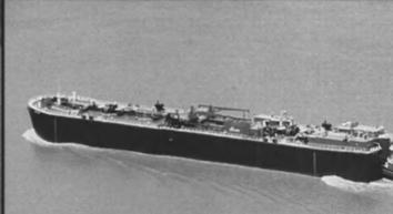
467 Foot Double Hull Tank Barge/127 Foot Tug
