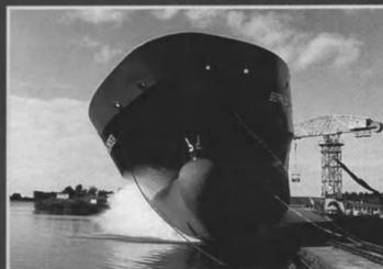
The Cono Feeder 200 containership *Bermuda Islander* being side-launched at Tille Shipyards in north Holland.
