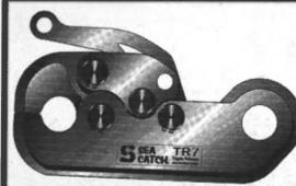
John McMillan Design developed the Sea Catch Toggle Release, a high-tech quick-release designed for safety during the release of a line under load. The product incorporates an old and proven toggle linkage principle, and is constructed from computer-generated parts, precision-cut from stainless steel plate.
