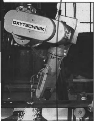
The Oxytechnik plasma system can cut plates up to 65 mm in thickness, and is equipped with a special design that allows cutting closer to the flanges.
