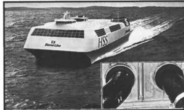
CSD sealing plug used on a new ferry under construction for Stena Line.
