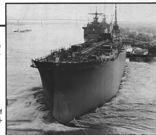
Pictured is the launching of the first of four double hull product/chemical carriers to be built by Avondale for AHL.
