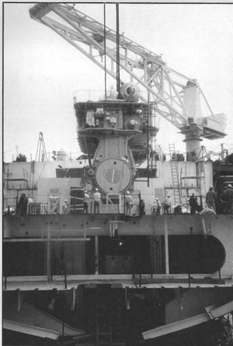
Despotico's MAN B&W diesel engine is lowered into place at Newport News Shipbuilding.
